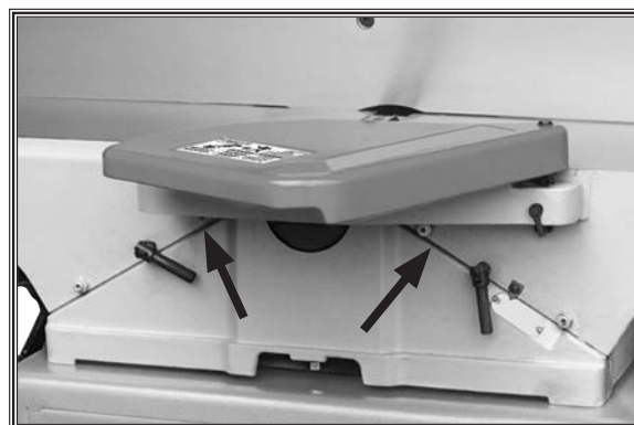
Figure 38. Location to lubricate table ways.
