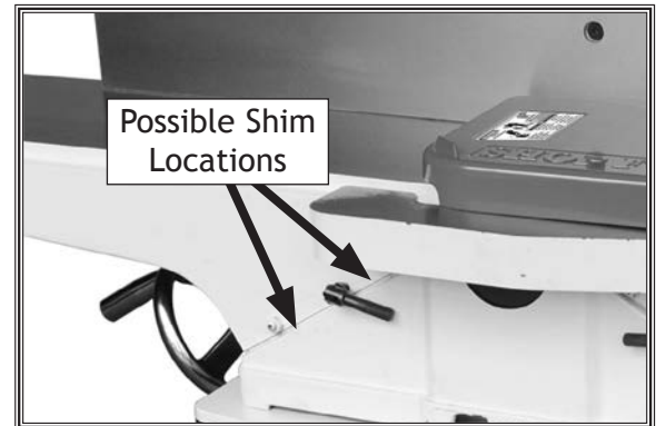
Figure 52. Locations to place shims when adjusting table parallelism.
