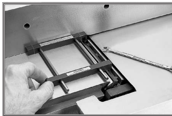
Figure 40. Setting knife height with a Jointer Pal®.
