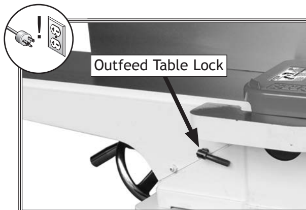
Figure 53. Location of outfeed table lock.
