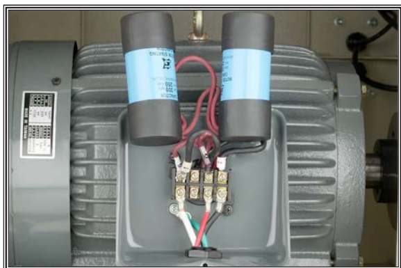
Figure 71. W1772 sanding drum motor wiring and start capacitors.
