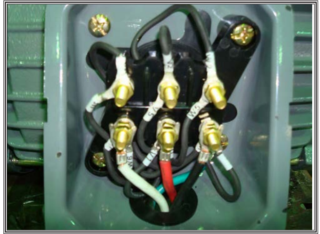
Figure 80. W1773 480V sanding drum motor wiring.
