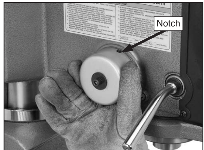
Figure 44. Adjusting spring tension.
