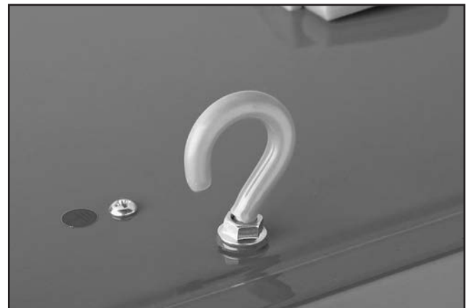
Figure 9. Machine hook installed.
