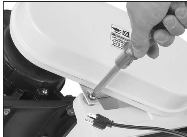
Figure 12. Installing pulley cover.
