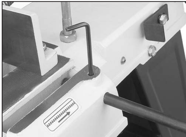
Figure 16. Installing work stop shaft.
