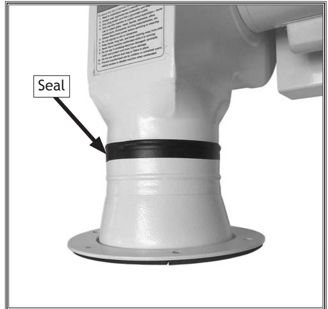
Figure 4. Duct tape wrapped around seam between collection flange and outlet.
